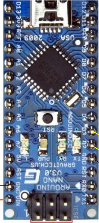
In Circuit Serial Programming (ICSP)
